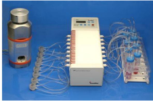
Figure 1: System set up in the 37° C room once the bone preparation was complete. Media was circumfused through the bone chamber and bone core without loss of nutrients or the excess build up of wast, with media changed every 2 days.
